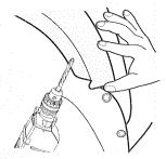
**b.** Place the fender trim in the desired installation position and drill a hole using the fender trim's precut holes as a template and guide.
